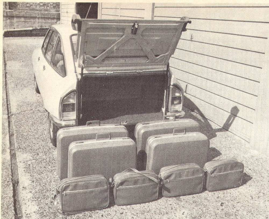
The unusual boot is a large symmetrical oblong hole, above, reached through a high-lifting tailgate supported by struts. The boot swallowed a respectable 10.4 cu. ft. of our test luggage, left
