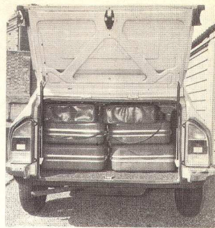
The unusual boot is a large symmetrical oblong hole, above, reached through a high-lifting tailgate supported by struts. The boot swallowed a respectable 10.4 cu. ft. of our test luggage, left
