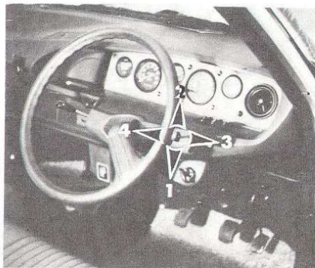
Fig. 16 - Right-hand drive Direction indicator/horn/ headlamp flasher switch 1 & 2 R.H. & L.H. wipers 3 Headlamp flasher 4 Horn
