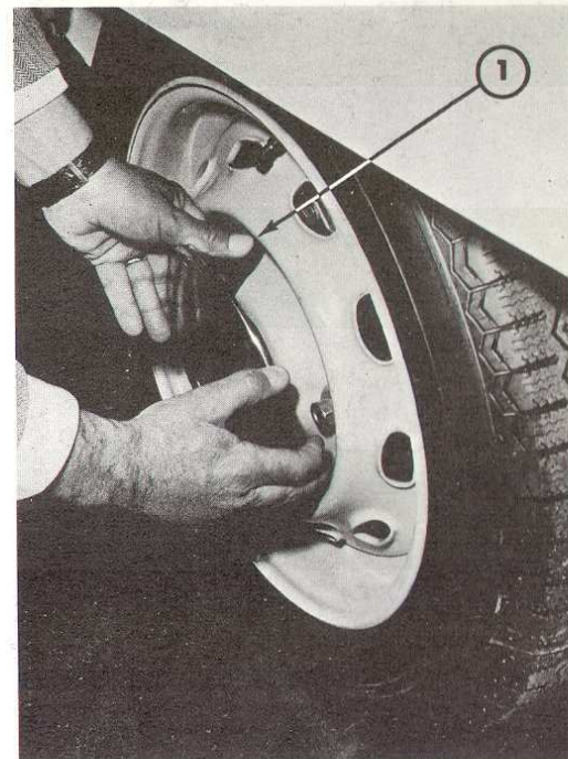
Fig. 31 – Refitting the hubcap 1 Hubcap leaf-spring
