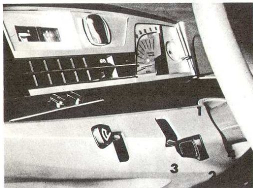
Fig. 16 - Left-hand drive Direction indicator/horn/ headlamp flasher switch 1 & 2 R.H. L.H. wipers 3 Headlamp flasher 4 Horn
