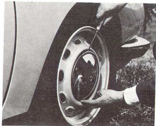
Fig. 30 – Removing the wheel hubcap
