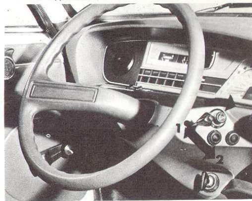
Fig. 18 – Right-hand drive Lighting control 1 Side/tail or main beam 2 Dipped beam
